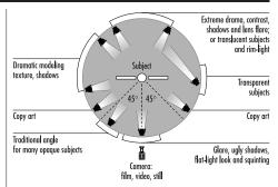
The oversimplified diagram above shows some of the ramifications of positioning lights for different subject types & lighting effects. The diagram is only useful as a starting point for new pros. All subjects & scenes are different and make different demands upon lighting. The height of the lights & camera, and the subjects angles & reflectivity must be considered.
