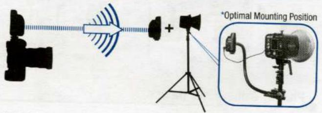
Camera with Plus® III in hot shoe (Transmitting)
