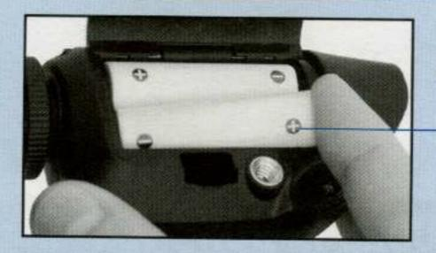
Note proper polarity when installing batteries.
