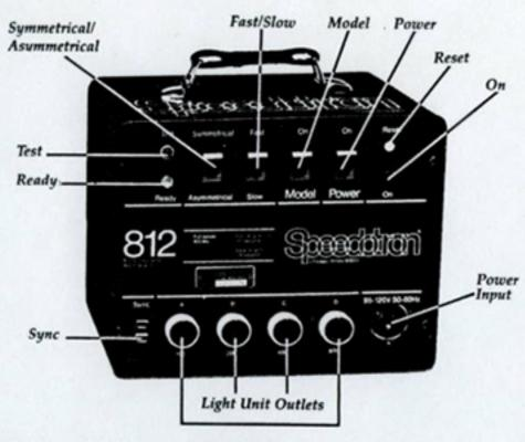
Power - turns power supply on and off (flashes light units when turning off).
